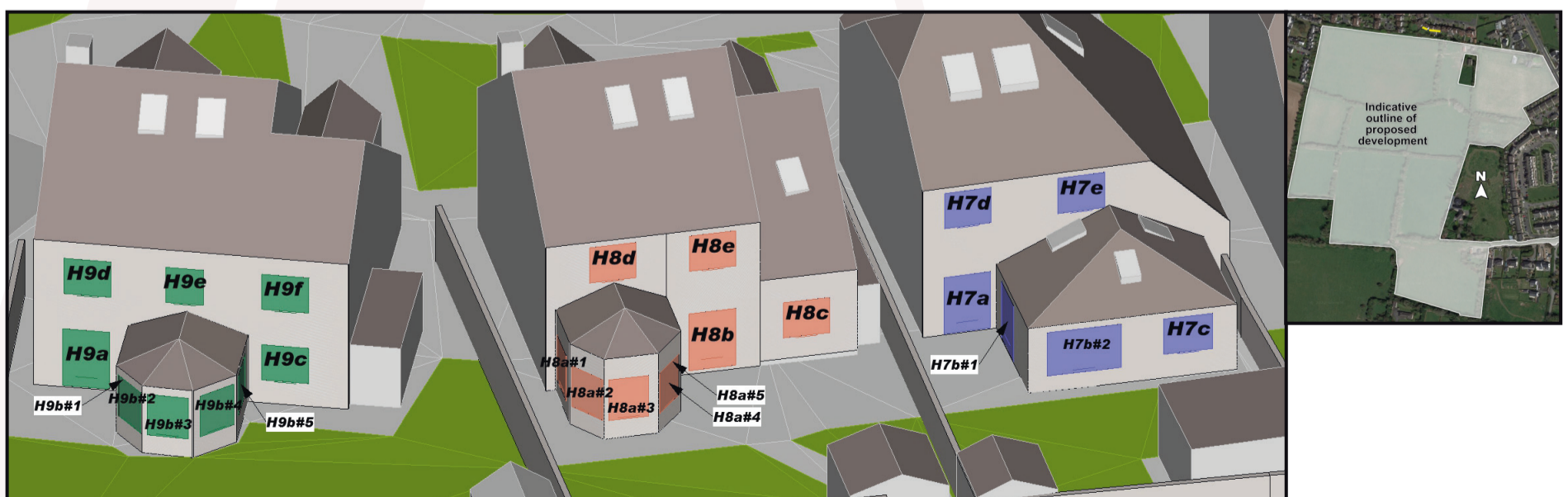
Figure 6.17: Highlighted areas indicate the position of assessed windows (L), Aerial view of assessed location (R)
