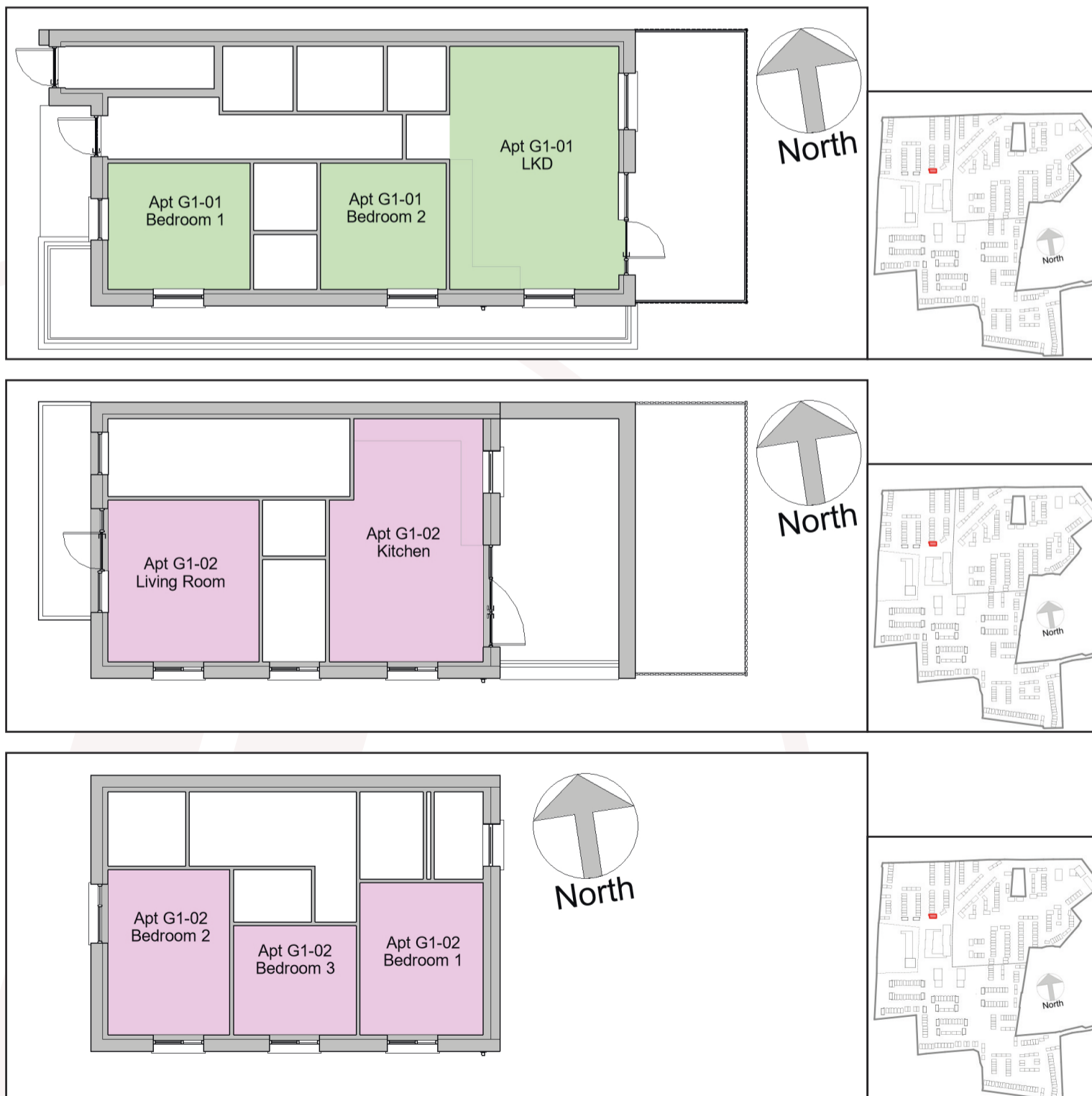
Figure 7.74: Floor plan of assessed building: Ground Floor (T), 1st Floor (M), 2nd Floor (B), Keyplan highlighting the assessed building (R).
