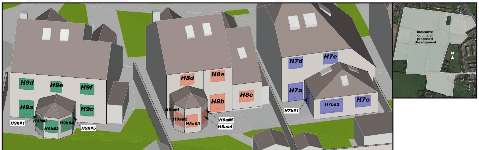
Figure 6.38: Highlighted areas indicate the position of assessed windows (L), Aerial view of assessed location (R)
